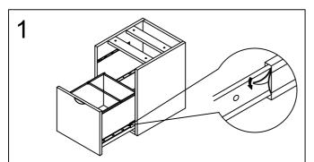
Remove drawer from pedestal. Fully open drawer. Where first slide meets second slide there is a small clip. Pull the clip on the left hand slide up, push the clip on the right hand slide down. Pull drawer out.
