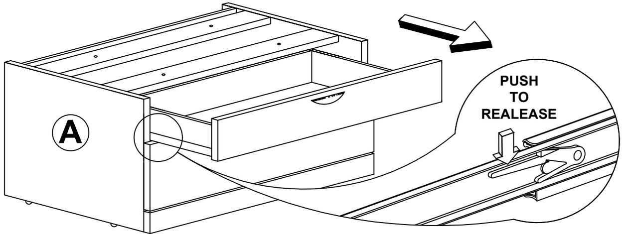
Push Drawer Slide at Drawer Box for PL1012(A). Push to release the Drawer Box and Pull Out from PL1012 body
