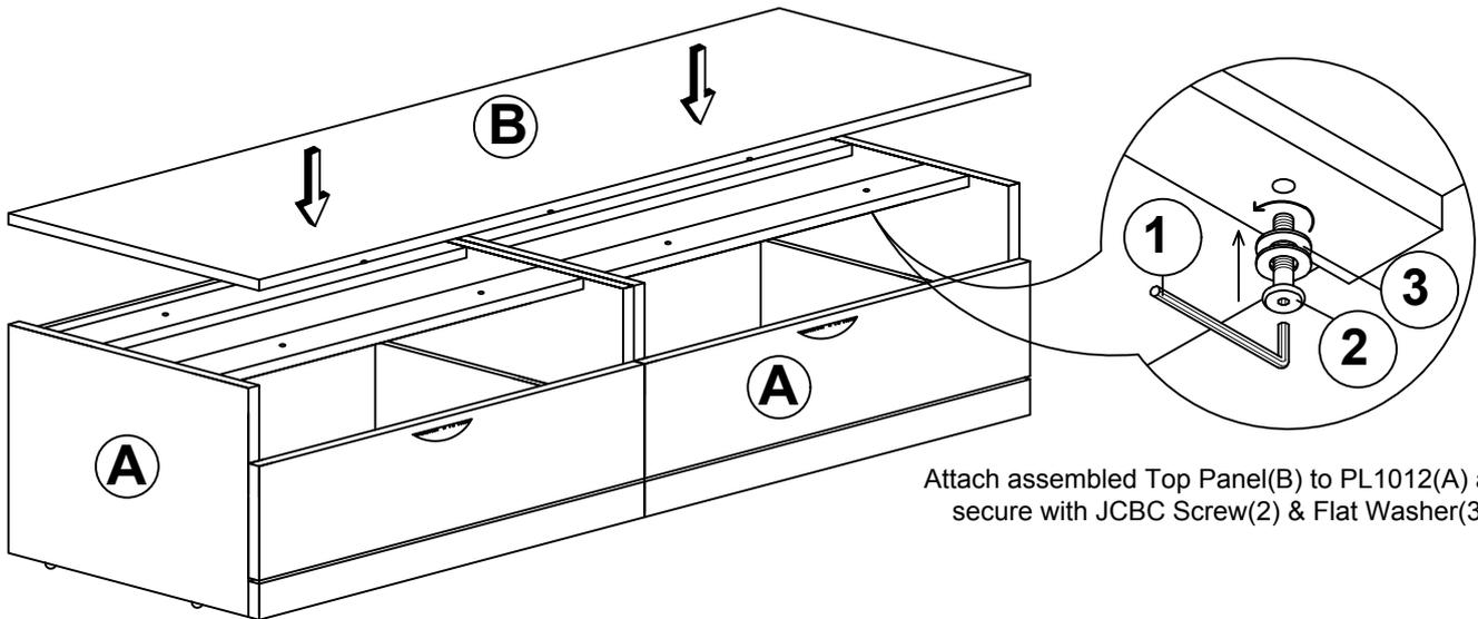
Attach assembled Top Panel(B) to PL1012(A) and secure with JCBC Screw(2) & Flat Washer(3)
