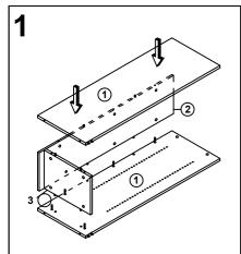
Attach Back Panel(2) & Bottom Panel(3) to Side Panel(1) by using Cam Lock(A) and Klix Cam(B).
