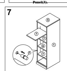
**Insert Shelve Support Pins(F)** into the pre drilled holes and place Adjustable Shelves(7) at convenient distances.
