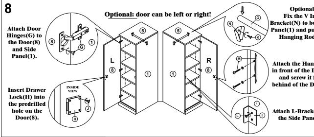
**Optional:** Fix the V Iron Bracket(N) to both Side Panel(1) and put in the Hanging Rod(O).
