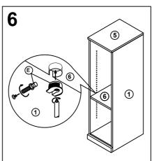
**Insert Center Shelve Pins(E)** into the pre drilled holes and place Fix Shelve(6) at convenient distances.
