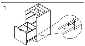
Remove drawer from pedestal. Fully open drawer. Where first slide meets second slide there is a small clip. Pull the clip on the left hand slide up, push the clip on the right hand slide down. Pull drawer out.
