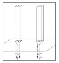
3. Attach top plate to center post using 4 MB\*40 bolts and 4 Locking Washer with allen key
