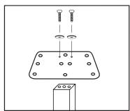
4. Attach top plate to wood top using 16 wood screws.
