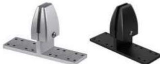
Dual mount – goes in between 2 face-to-face work surfaces. Cut outs wrap around a 1" thick surface. Screws from the underside. No need for holes in the top of the desk. Must have an overhang to work.
