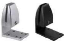
Single mount – wraps around a 1" thick surface. Screws from the underside. No need for holes in the top of the desk. Must have an overhang to work.
